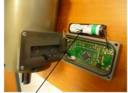
Use a AA 3,6V Li-SOCL2 battery Reposition the wires correctly before tightening the 4 screws
